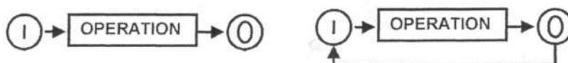
Figure 1a (left) and Figure 1b (right). Mere input-output analysis (left) versus feedback loop (right).
